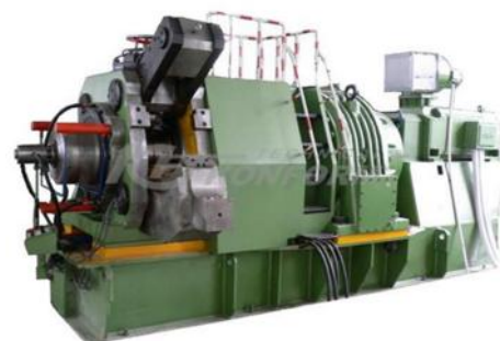
Figure 3. Conform. Left: equipment. Right: deformation scheme.
