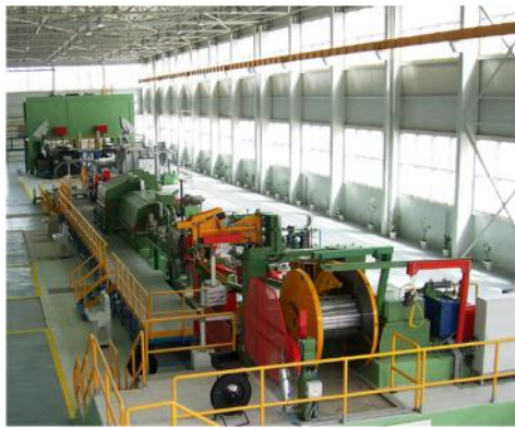
Figure 1. Continuous casting and rolling. Left: equipment and layout. Right: deformation scheme.
